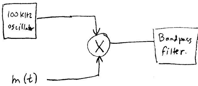
The ring modulator is used as a switching modulator, which generates odd harmonics.
