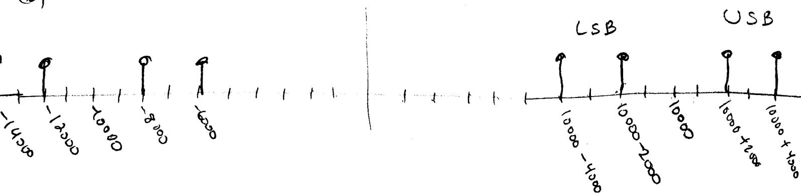
$m(t)$  is already a modulated signal, with components at  $2000$  ( $\omega_2 - \omega_1$ ) and  $4000$  ( $\omega_2 + \omega_1$ ).
