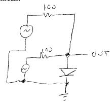
Apply 100 kHz and 1 kHz sine waves at .5 volts p-p each. Show the waveform and spectrum. Show the frequency ranges of 90 kHz to 110 kHz, and 0 to 10 kHz. Increase the signals as before, and show the spectrum at 1,2, and 10 volts p-p input. Which components are non-harmonic? Comment on what you see.
