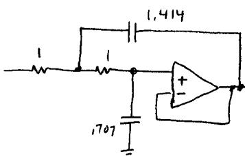
Design for 1 kHz,  $D = 1.414$ ,  $R_1 = R_2 = 10K$ .
