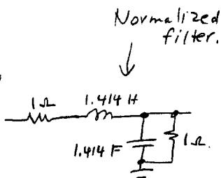
Scale Frequency — divide L and C by w
