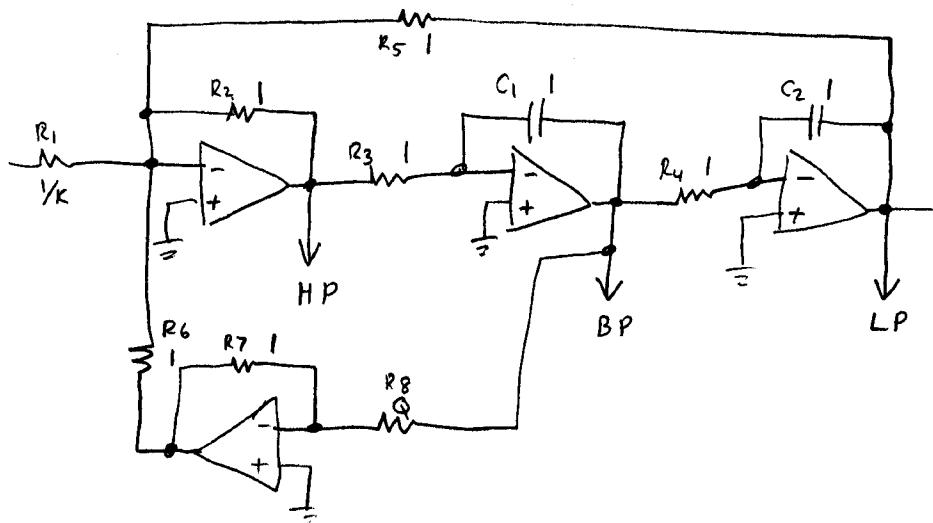
$$Q = \frac{R_8}{R_7} \quad \omega_0 = \frac{1}{R_3 R_4 C_1 C_2}$$
