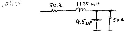
(checked with simulator  $-9 \text{ dB}, -90^\circ @ 1 \text{ kHz}$ )  $40 \text{ dB/dec}$
