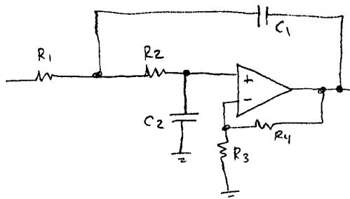
$$\frac{V_{out}}{V_{in}} = \frac{K}{s^2(R_1R_2C_1C_2) + s(R_1C_2 + R_2C_1 + R_1C_1(1-K)) + 1}$$
