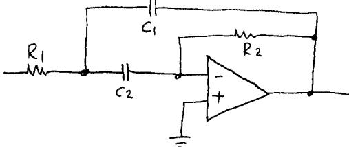
$$\frac{V_{out}}{V_{in}} = \frac{-s(R_2C_2)}{s^2(R_1R_2C_1C_2) + s(R_1C_2 + R_2C_1) + 1}$$
