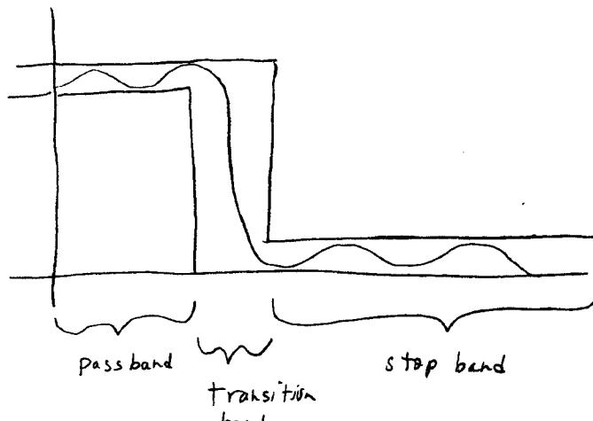
→ Gain or loss in pass band must be between certain limits.
