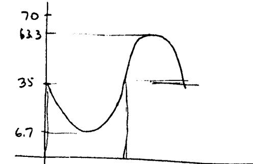
Current is the load current, halfwave rectified
