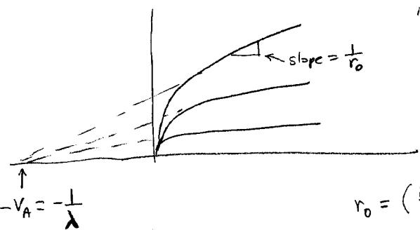
$$r_o = \left( \frac{\partial i_D}{\partial V_{DS}} \right) \Big|_{V_{GS}=\text{const}}$$
