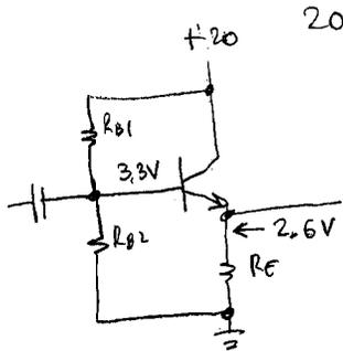
Direct couple to next stage, eliminating its bias resistors.
