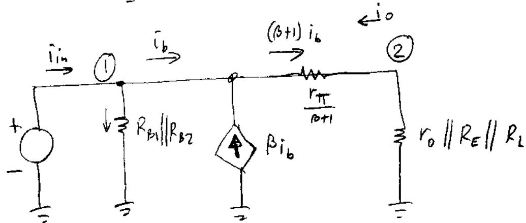
$$\frac{V_2}{V_1} = \frac{r_o || R_E || R_L}{\frac{r_T}{\beta+1} + r_o || R_E || R_L} \approx 1 \quad (\text{a little less})$$
