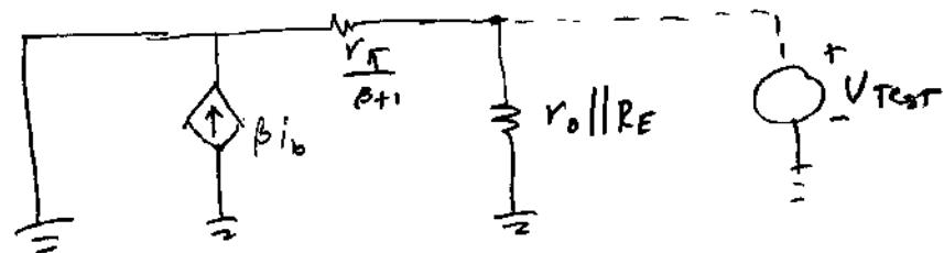
$$\text{For shorted input} -- r_o \parallel R_E \parallel \frac{r_\pi}{\beta+1} \approx \frac{r_\pi}{\beta+1}$$
