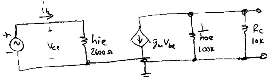
$$\text{Gain} = g_m R_L \quad \text{where } R_L = \frac{1}{h_{oe}} \parallel R_C$$
