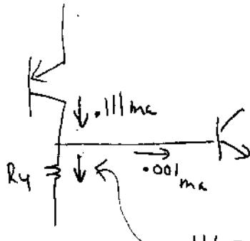
$$.111 - .012 = .099 \text{ mA} \quad V_{R4} = IR = (.099)(16 \text{ k}) \\ = 1.58 \text{ V. } \approx 1.6$$
