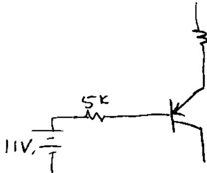
If  $V_2 = 11V$ , then  $V_3$  must be 11.6V.
