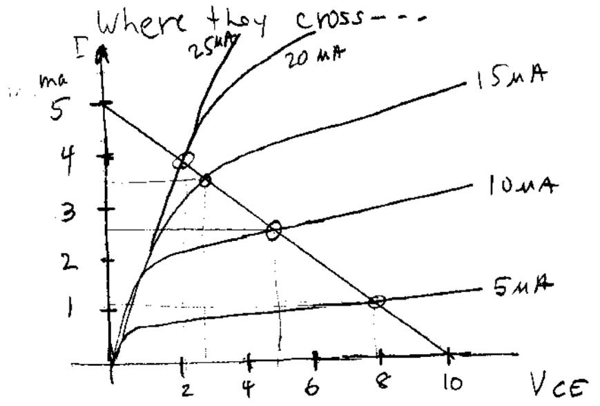
Transistor:  $I_C$  vs.  $V_{CE}$
