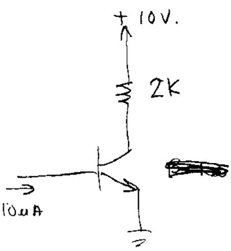
Plot transistor curve and load line on same graph -
