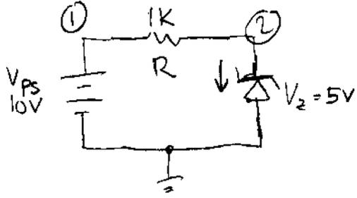
$$I = \frac{V_{ps} - V_z}{R} = \frac{5}{1K} = 5 \text{ ma}$$
