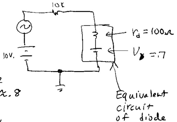
Equivalent circuit of diode
