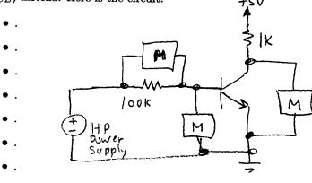
Adjust the base supply in steps to get the same base currents  $(I_B)$ as you had in the previous section. The other measurements associated with the base  $(V_{RB}, V_{BE})$  should be the same, too, or very close. Don't worry if they change a little.
