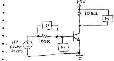
Fill in this chart. Adjust the base power supply to achieve the desired collector current  $(I_C)$  as measured on the meter. Then read  $V_{BE}$  (base to emitter voltage) from its meter. Then determine  $I_B$  (base current) indirectly by measuring the voltage across the series base resistor.
