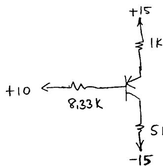
$$\begin{aligned} R &= R_1 \parallel R_2 = \frac{(10k)(50k)}{10k + 50k} \\ &= \frac{500 \text{ Meg}}{60k} \\ &= \frac{50}{6} \text{ k} \\ &= 8.33 \text{ k} \end{aligned}$$
