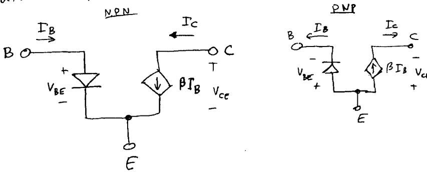
Substitute the model for the transistor, and analyze.
