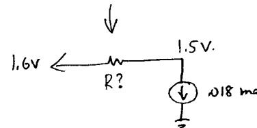
$$R = \frac{V}{I} = \frac{1.6 - 1.5}{.018 \text{ ma}} = \frac{.1}{.018 \text{ ma}} = 5.5556 \text{ K}$$
