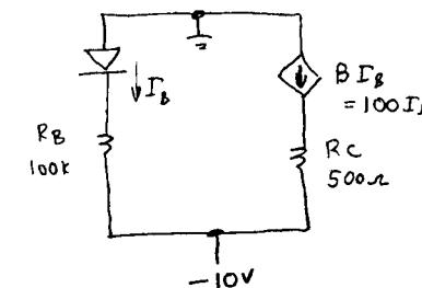
$$V_{RB} = 9.4 \quad I_B = \frac{9.4}{100k} = .094 \text{ mA}$$
