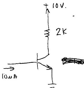
Plot transistor curve
