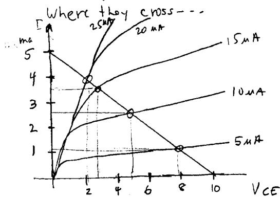
Transistor:  $I_C$  vs.  $V_{CE}$
