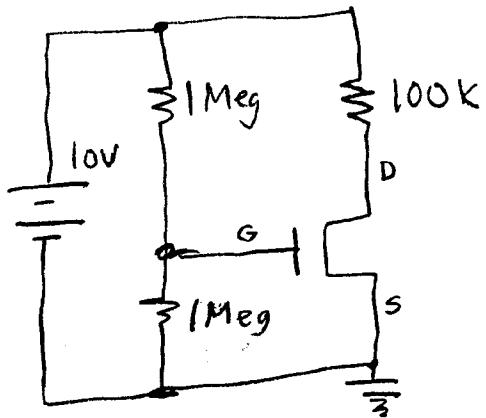
Here's the equivalent circuit:
