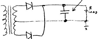
It charges when the diode is on, then holds the charge.
