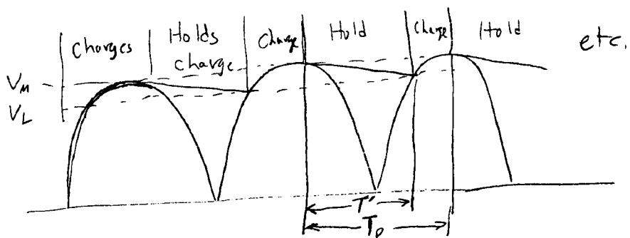
The capacitor holds the voltage to nearly the peak voltage.
