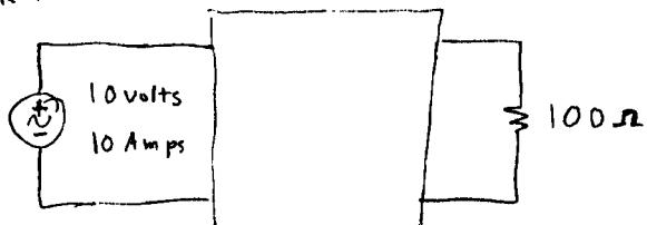
The source (10 Volts) can supply 10 Amps - (100 watts)
