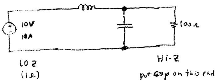
$$\begin{aligned} \text{pick value of cap for } X &= \sqrt{Z_1 Z_2} \\ &= \sqrt{(1)(100)} \\ &= \sqrt{100} \\ &= 10\ \Omega \end{aligned}$$
