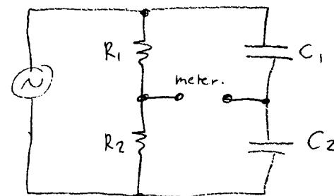
in balance when  $\frac{R_1}{R_2} = \frac{C_2}{C_1}$
