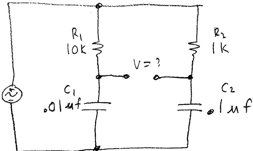
$$V = 0 \text{ when } \frac{R_1}{C_1} = \frac{R_2}{C_2}$$
