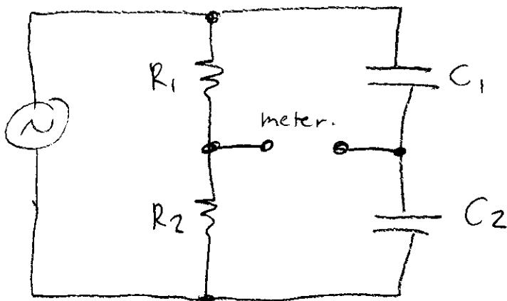
in balance when  $\frac{R_1}{R_2} = \frac{C_2}{C_1}$
