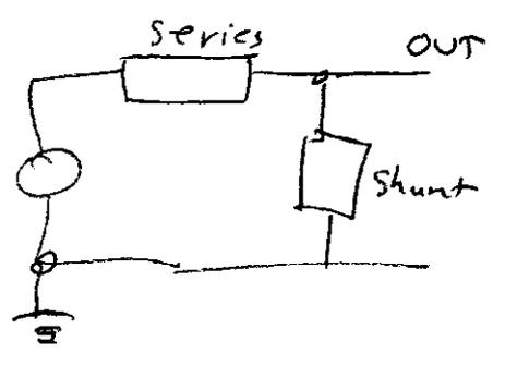
$$= V_{IN} \frac{1}{j^2 \omega^2 LC + 1} = \frac{1}{-\omega^2 LC + 1}$$
