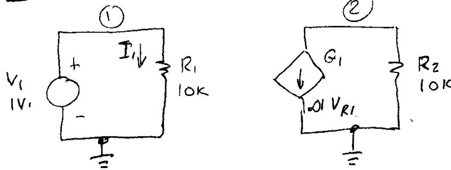
$$\text{Node } 2 : G_1 V_1 + \frac{V_2}{R_2} = 0$$
