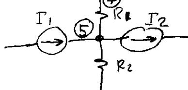
$$I_1 - I_2 + \frac{V_4 - V_5}{R_1} + \frac{-V_5}{R_2} = 0$$
