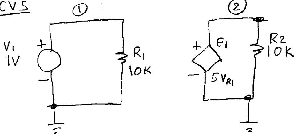
$$V_2 = 5 V_{R1} = 5$$
